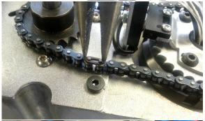
Wrap the new Chain around both sprockets, install Master Link and clip using Needle Nose Pliers
