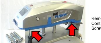
Remove three #8-32 x 3/4" Screws from Control Housing using Short #2 Phillips Screwdriver
