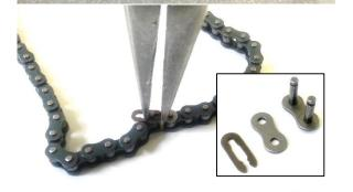
Remove Master Link from new Chain using Needle Nose Pliers
