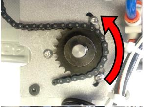
Use the new Chain to rotate smaller sprocket counter-clockwise until it stops
