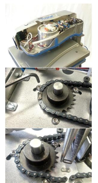
Lift off Control Housing and lay it gently on left side of press
